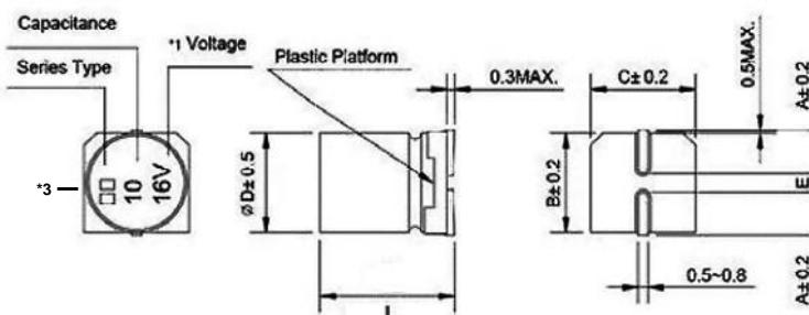
\*1 Voltage mark for 6.3V is [6V] or [6.3V]    \*3 Surface Marking Types: jbN, jN, CN
