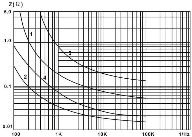
Fig.3 Typical impedance as a function of frequency
