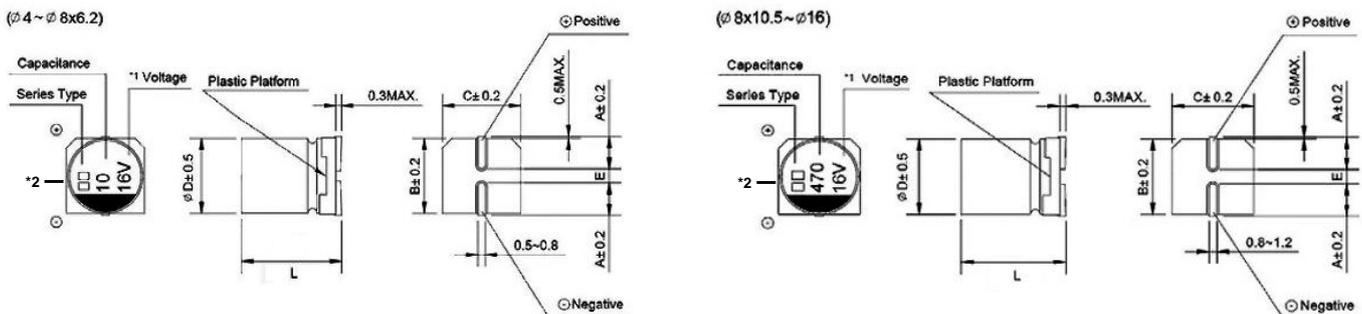
\*1 Voltage mark for 6.3V is [6V] or [6.3V] \*2 Surface Marking Types: jbE, jE, EL, VL
